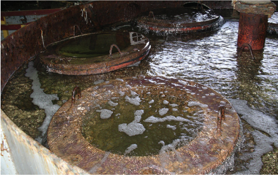
The gold bearing cyanide solution on the top of an ion exchange column.
